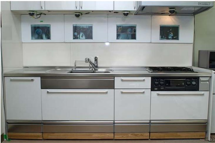
**Fig. 1.** Overview of the “Kitchen of the Future.” Video cameras, and microphones, LCDs, and foot switches are installed under the cupboard, on the wall, and on the floor, respectively.
