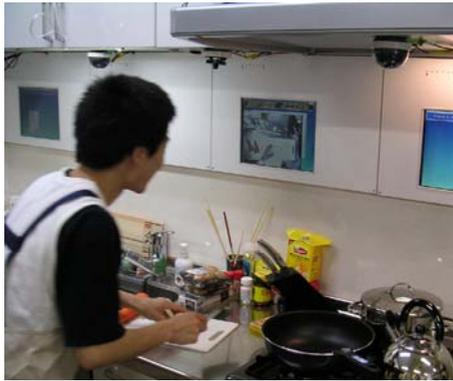
**Fig. 4.** A user is cooking while replaying the recorded pictures and sounds of the cooking process on the LCDs. The images are displayed on one of the four LCDs at the workplace. When he completes the displayed step, he can view the next step by pressing the foot switch.
