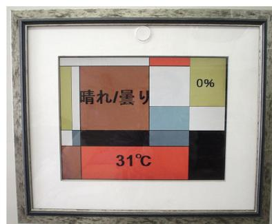
**Figure 1. A framed LCD displays the weather forecast as distributed on the Internet, with animation (above) and color blocks(below). When a human approaches the display, additional literal information will appear.**
