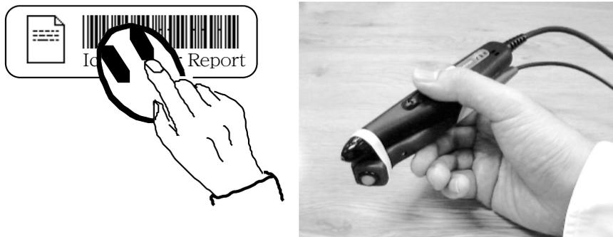
Figure 4: When the bar code part of the IconSticker is scanned with a mouse equipping with a bar-code reader, the original computer icon is opened on the display (left). A combination of a mechanical pen-mouse and a bar-code wand is used in the current prototype (right).
