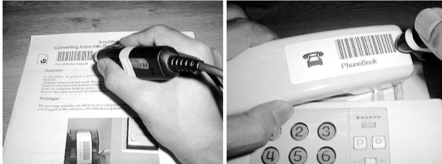
Figure 5: Examples of IconSticker applications. It can be used to find the original soft copy (left), or to access a telephone database (right).
