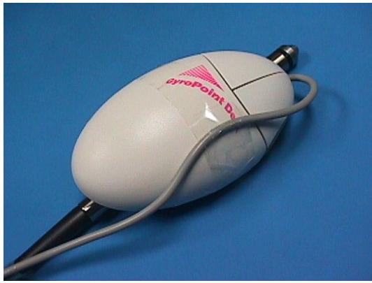
Figure 2: FieldMouse#2: Combination of a barcode reader and a gyro-mouse.
